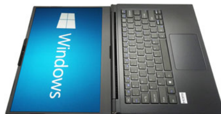
Figure 5 - LCD Panel Open to 180 degrees with Screen Rotated
